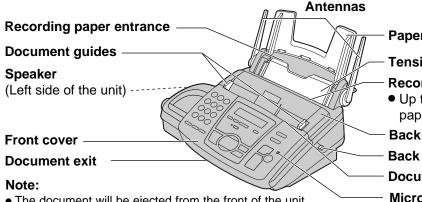
• The document will be ejected from the front of the unit. Install the unit on a desk or floor with a smooth surface and do not place anything in front of the unit.
